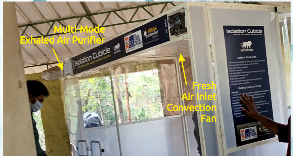
Multi-Mode Air Purifier to treat patient's exhaled air Fresh Air Convection fan for Patient's comfort
