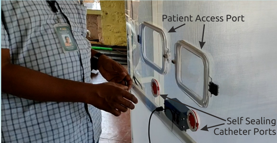
In-built Dual Patient Access Ports and Dual Self Sealing Catheter Ports
